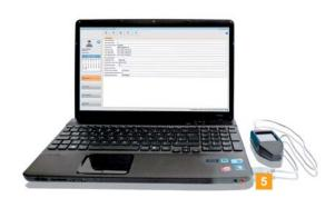
5 If possible, leave the DLKPro plugged into the computer when you finish working with it – this will charge the integrated rechargeable battery e. g. for the next card download.
